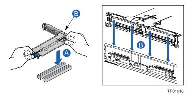
Figure 33. Installing the PCI Riser Assembly into the Chassis
